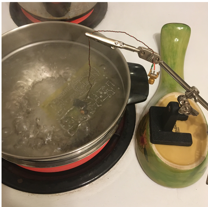
Figure 6.0.9: Boiling of entire circuit in pot of water on the stove to anneal inductor.
