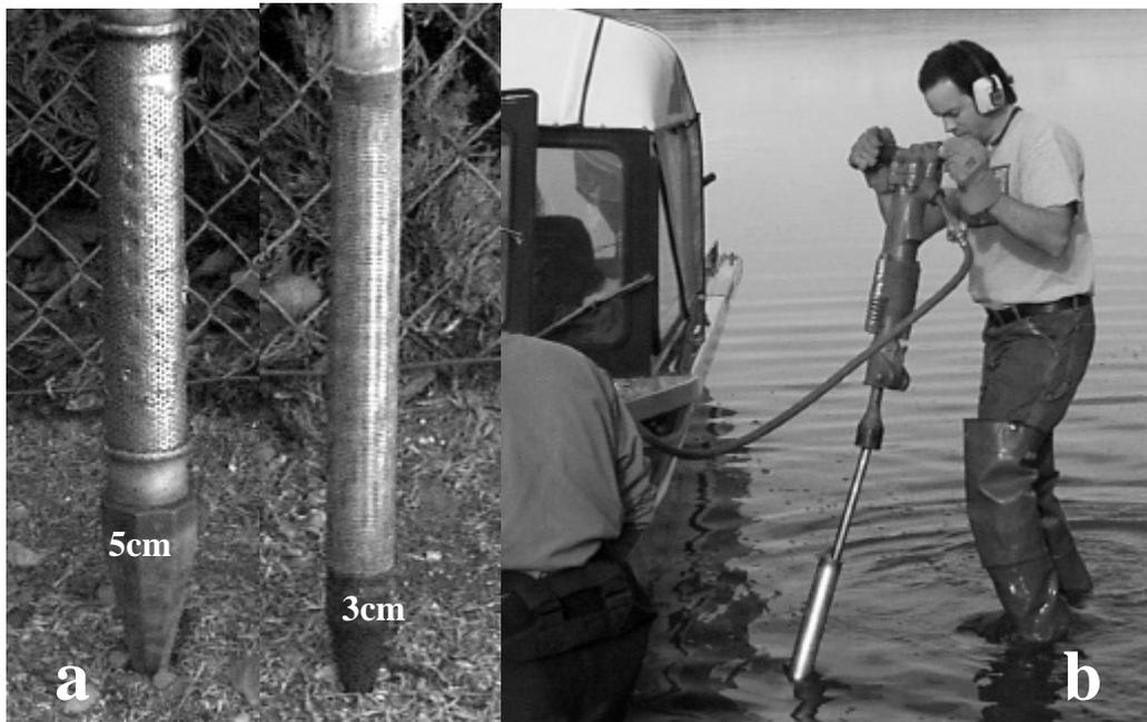
Figure 13: Galvanized piezometers and their installation. (a) Galvanized piezometers had an inside diameter of either 5.0 cm or 3.0 cm. (b) Installation of a Midwest piezometer using a pneumatic hammer.
