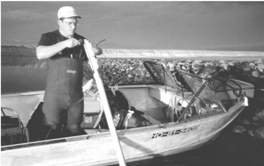
Figure 15: Slug test pressure regulating device with pressure transducer lowered inside to record head response vs. time. The Columbia River undercuts the Ringold Formation in the background, exposing ancient alluvium in an area now known as the White Bluffs.
