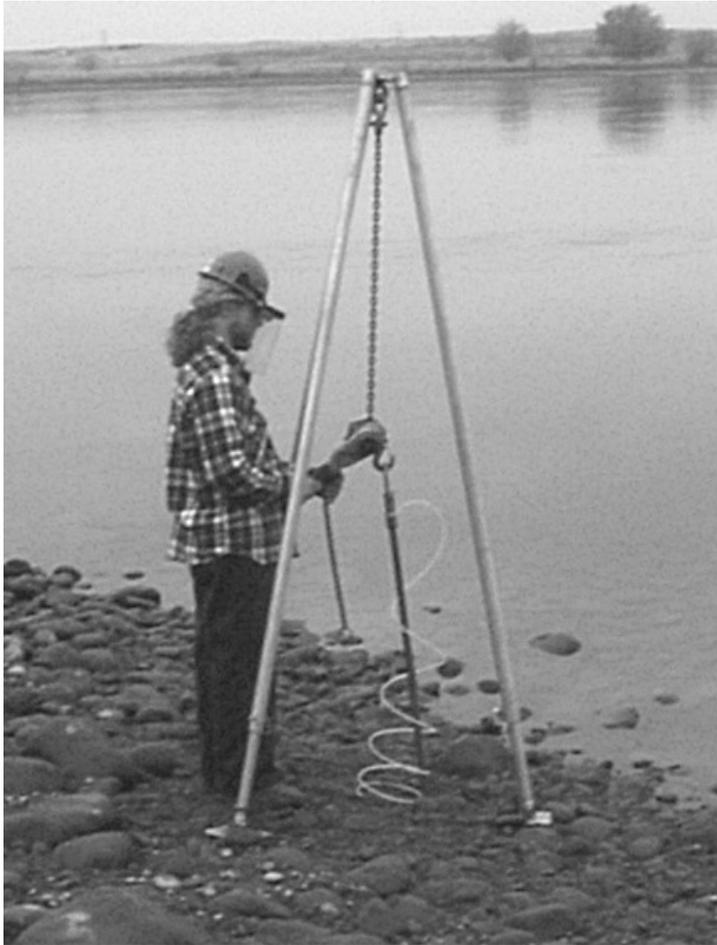
Figure 11: Piezometer extraction equipment used to remove the Geoprobe<sup>®</sup> driving system.
