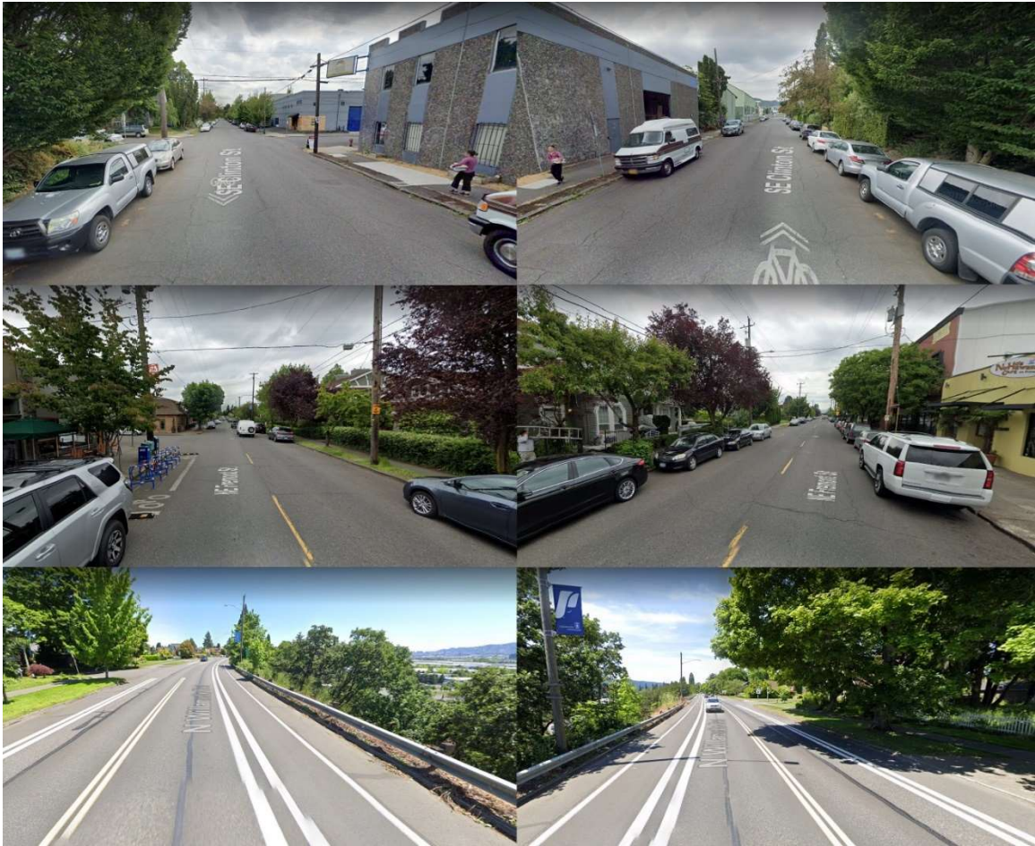
Figure 4.2 Bicycle infrastructure examples, from top to bottom: shared bikeway, no bicycle facilities, and bicycle lanes with a marked buffer.
