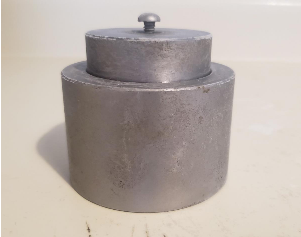
Figure 2.6: Steel (4140 ACRALLOY tool-grade, quenched and tempered) mold and piston device used for 1-D compression testing of soil specimens, seated.
