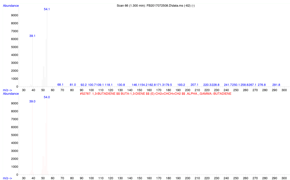
Figure 8.9: Mass spectrum of 1,3-butadiene (top, grey) compared to NIST library mass spectrum (bottom, red).
