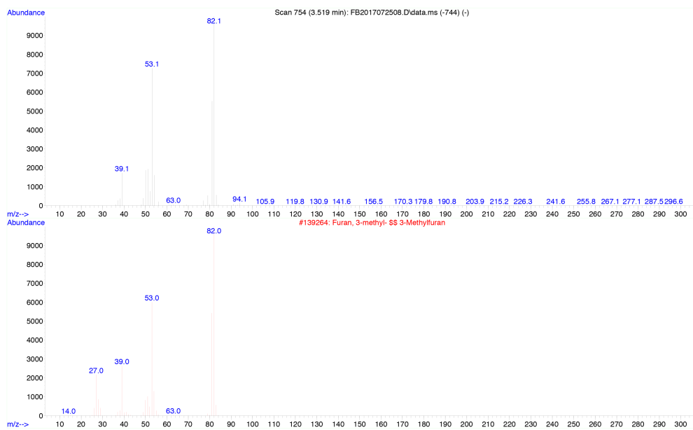
Figure 8.13: Mass spectrum of 3-methyl furan (top, grey) compared to NIST library mass spectrum (bottom, red).
