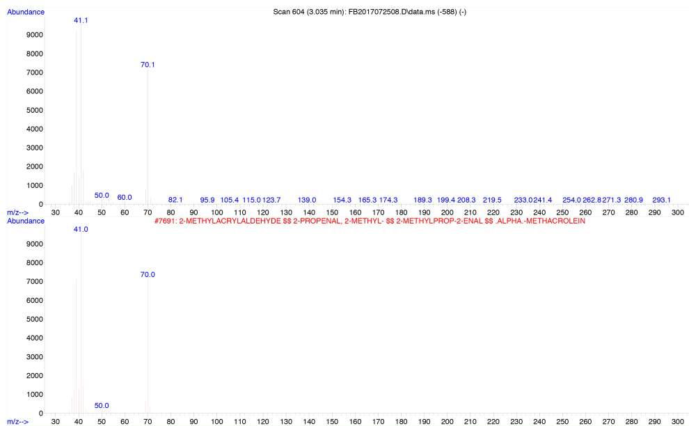
Figure 8.11: Mass spectrum of methacrolein (top, grey) compared to NIST library mass spectrum (bottom, red).
