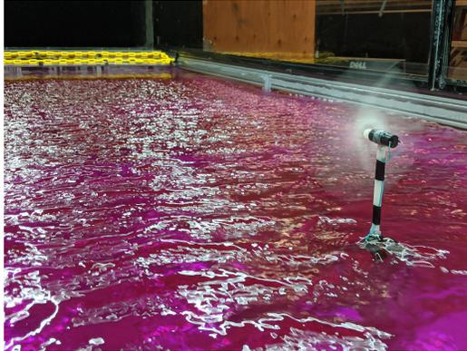
Figure 3: Photograph of the experimental setup with long-period waves and super-imposed wind generated waves.
