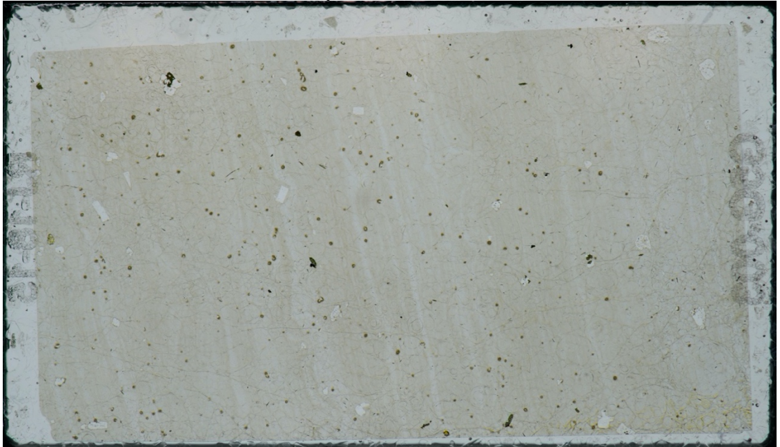
Figure 73. Thin section of glassy Bannock Ridge rhyolite, sample RJ-18-15, in plane polarized light.
