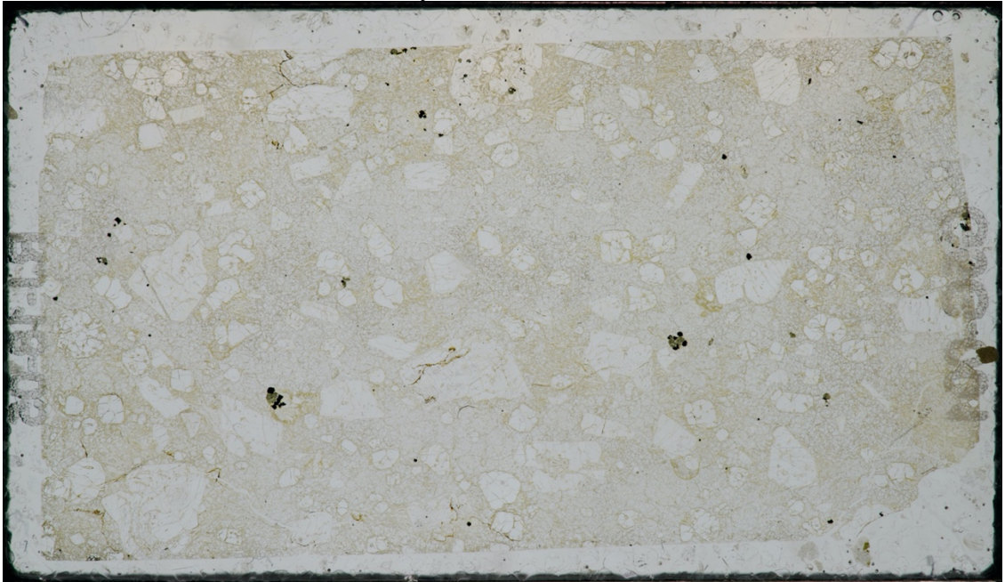
Figure 69. Thin section of 'Rhyolite SE of Round Mtn', sample RJ-18-05, in plane polarized light.
