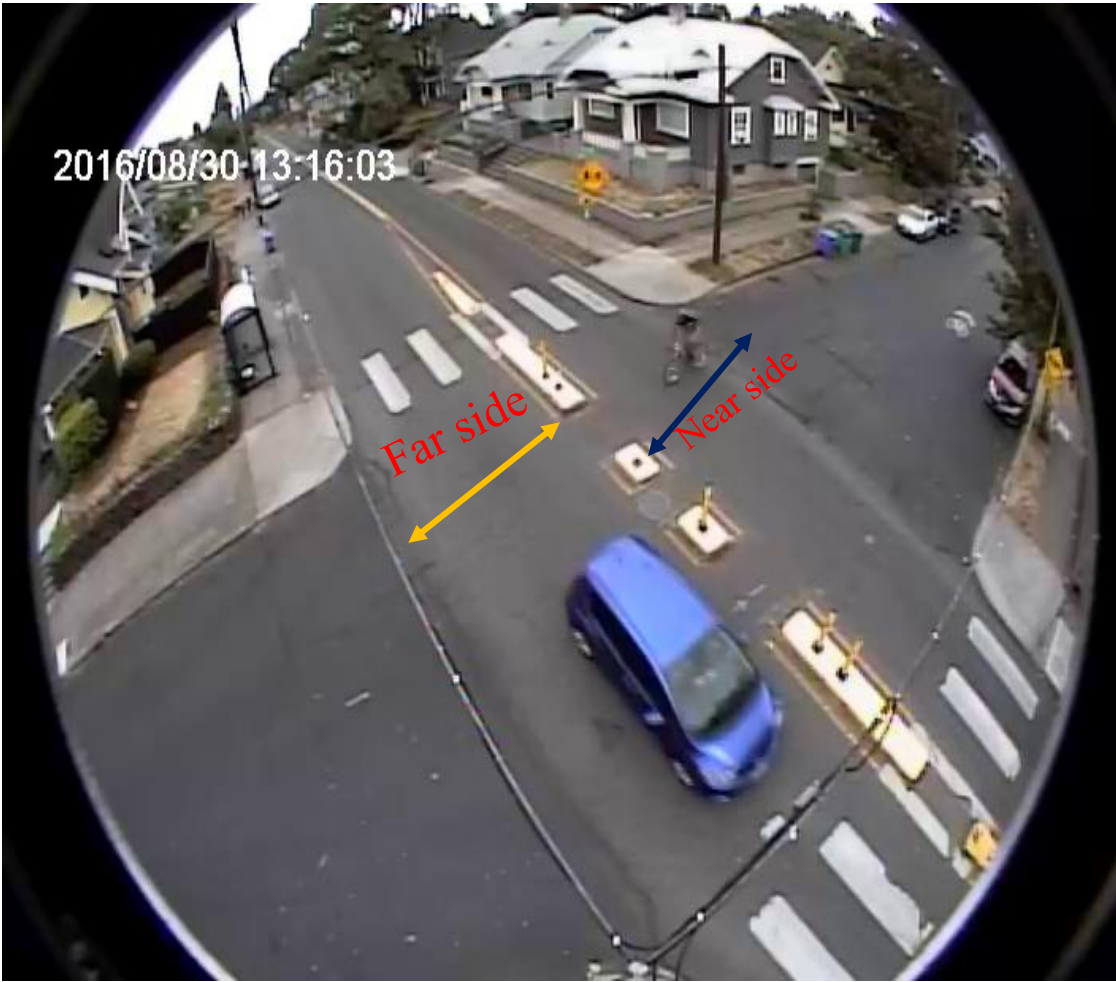
Figure 12: Plan view of NE Going & NE 15th Ave illustrating near and far sides for a bicycle crossing.
