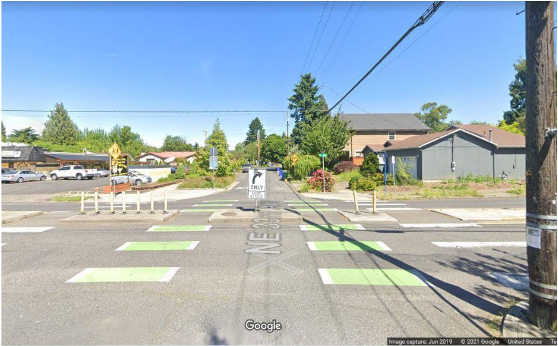
Figure 1: Typical intersection with cross-bike pavement markings. Source: Google Maps
