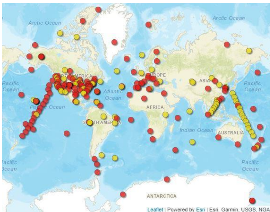
Figure 4.2: A map of atmospheric methane surface flask measurement sites as provided by NOAA ESRL GML. Red circles indicate active measurement sites and yellow circles indicate discontinued sites.
