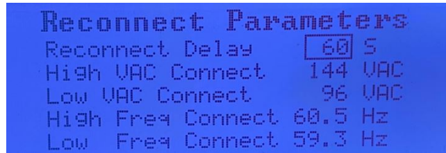
Figure 5.16: Time delay setting before inverter export power.
