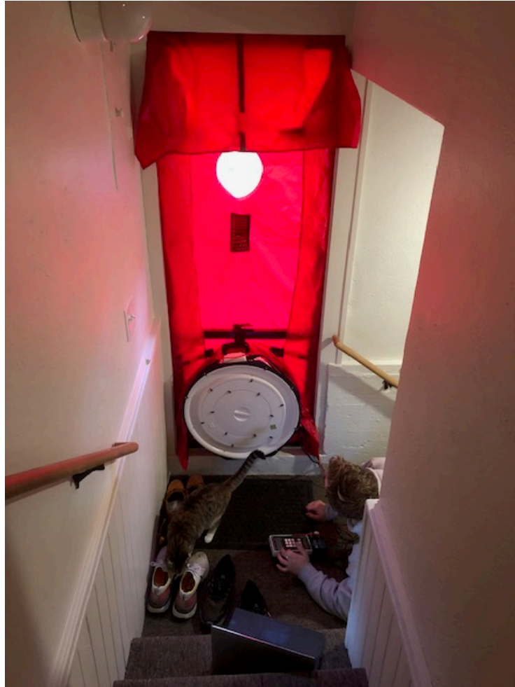
Figure 1. Blower door test set-up for envelope air tightness measurements.
