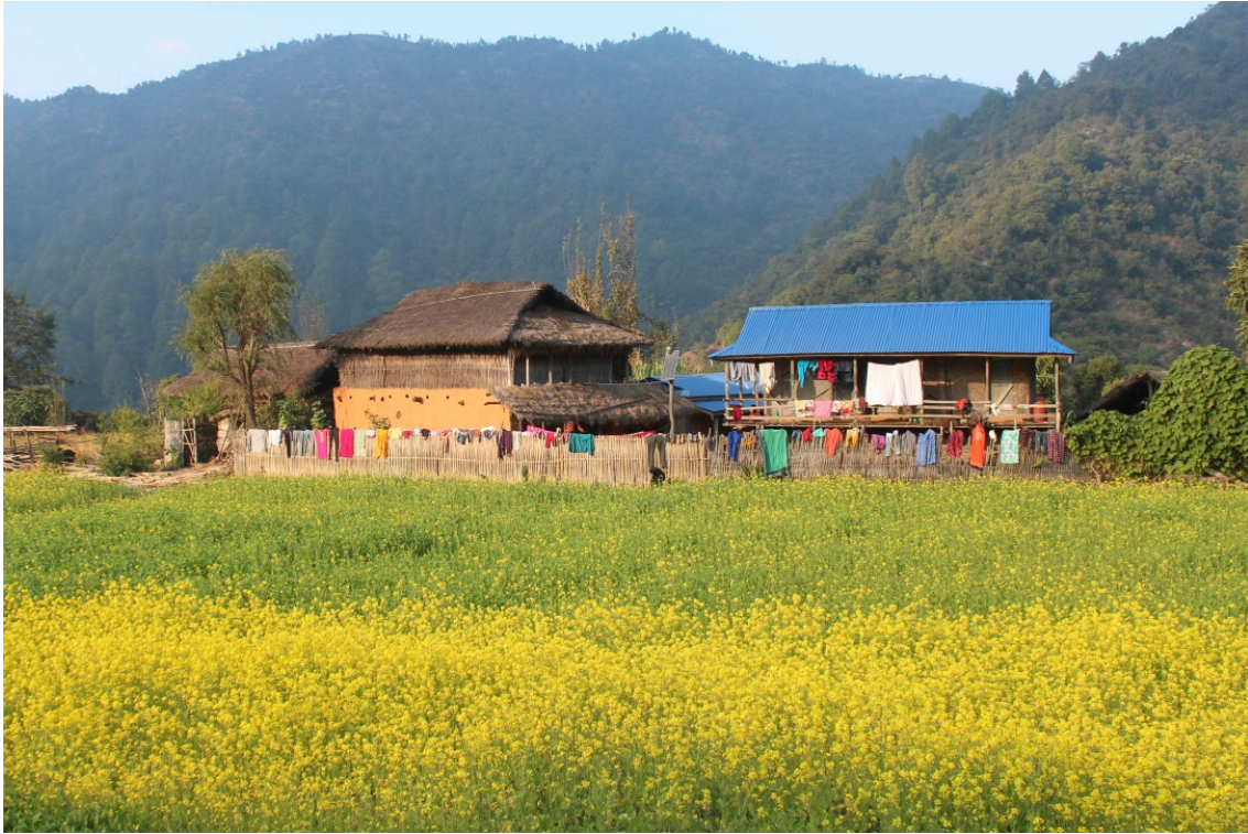
Figure 15: Examples of typical houses in the part of Rautamai Gaunpalika where I did research. The ground floor of the house on the left is constructed from stone and mud plaster, and the upper floor is made of bamboo. The roof is thatch. On the right, the house is made from wood, with a CGI roof. Both homes have a wooden frame. Note these are not the homes of research participants. Late fall, 2018.
