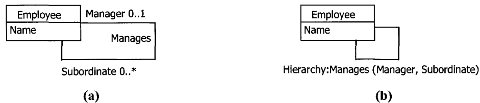
Figure 4.29: Example application of relationship patterns. (a) A hierarchy of manager and subordinates; (b) The hierarchy of manager and subordinates modeled after a relationship pattern called Hierarchy
