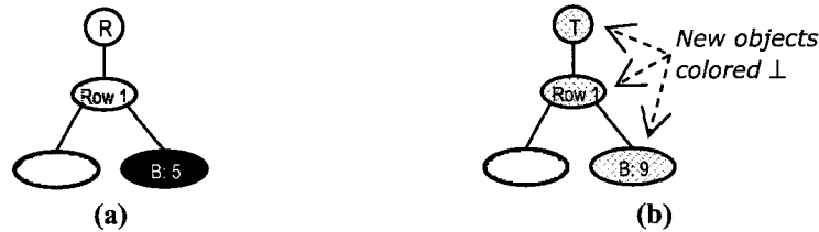
Figure 8.6: An illustration of data provenance. (a) A tree model of a relation R(A, B) with one tuple in the relation instance; (b) A model of the result of the query SELECT A, 9 AS B FROM R . The name T for the result table is chosen arbitrarily
