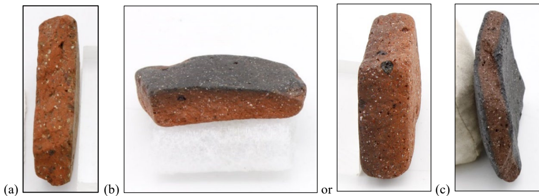
Figure 14. Margin types: (a) showing no distinct margins between the core (JF60); (b) margins fade into the core under the dark gray glaze (JF22 or JF319); (c) core and margins have distinct line between them (JF111).
