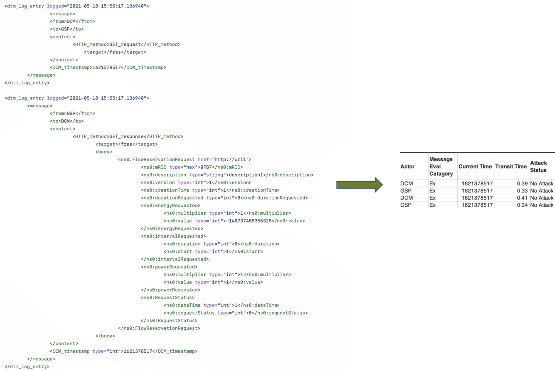
Figure B.1: XML to CSV conversion executed by the Trust Model Classifier
