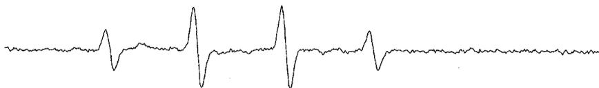
a) Fenton's reaction, after 5 min incubation:  $[H_2O_2] = 0.2 \text{ mM}$ ,  $[FeSO_4] = 0.05 \text{ mM}$ ,  $[DMPO] = 80 \text{ mM}$
