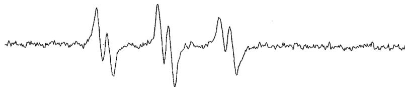
a) Fenton's reaction, after 5 min incubation:  $[\text{H}_2\text{O}_2] = 0.2 \text{ mM}$ ,  $[\text{FeSO}_4] = 0.05 \text{ mM}$ ,  $[\text{PBN}] = 50 \text{ mM}$
