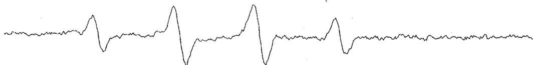
e) GSH oxidation by PN, after 5 min incubation:  $[PN] = 0.8 \text{ mM}$ ,  $[GSH] = 3.0 \text{ mM}$ ,  $[DMPO] = 80 \text{ mM}$ , pH 7.4
