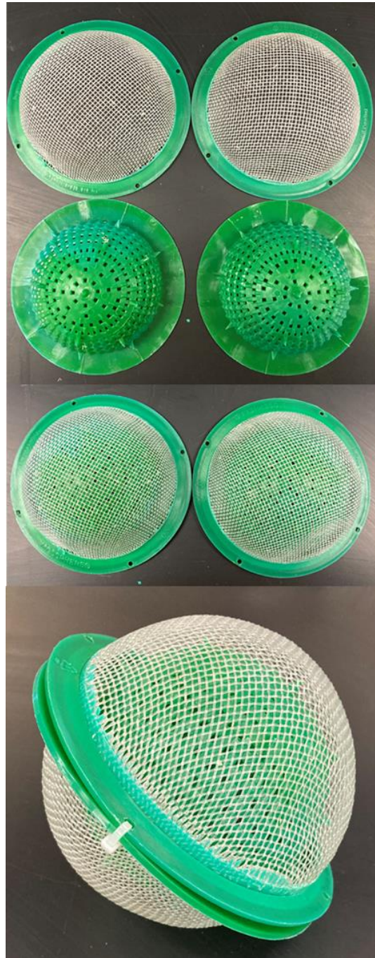
Figure 3. Mossphere design and assembly
