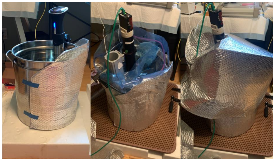
Figure S10. Insulation for heated bath. Progression of insulating the pot and submerging the microscope, from left to right.
