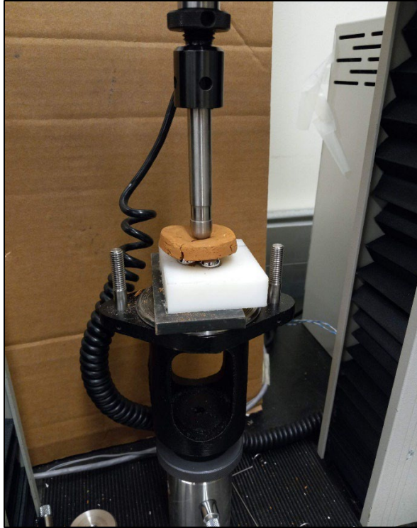
Figure 10. Ball-on-three-ball testing apparatus.
