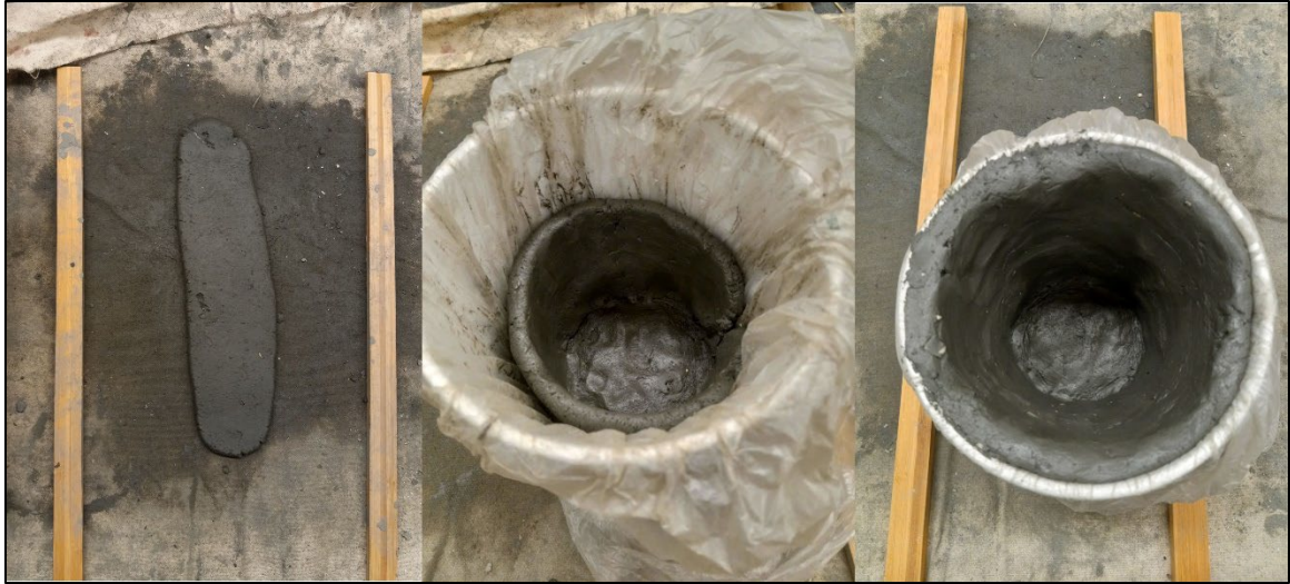
Figure 14. From left to right: clay slab after being rolled out on 1 cm rollers, molding the base and sides of vessel in plastic-lined pot, and finished vessel before drying.
