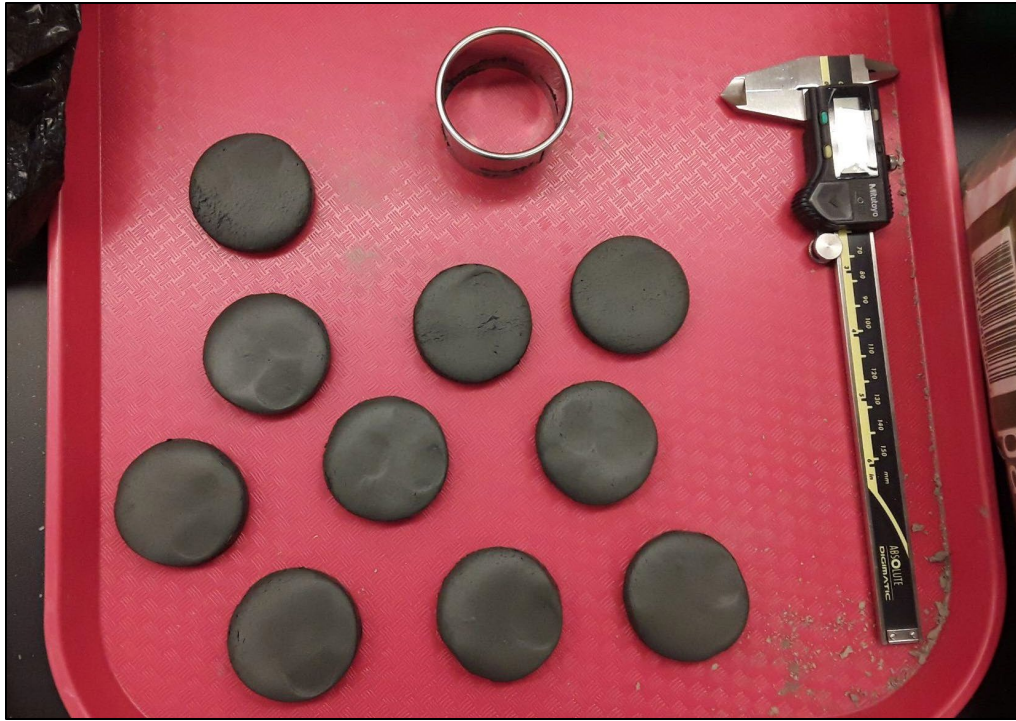
Figure 8. Unfired test tiles showing the cutter used to make them equal sizes.
