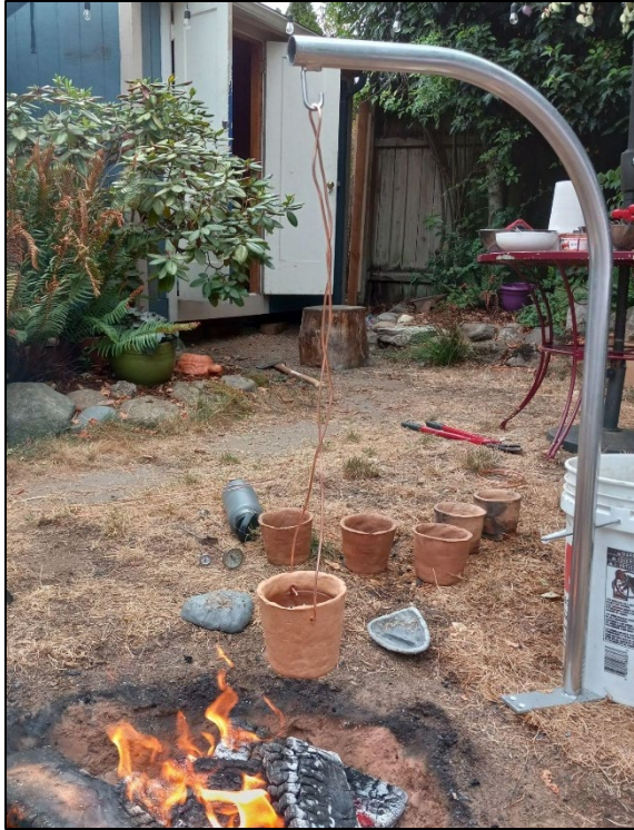
Figure 18. Norton style replicated pot during suspended heat trial, showing suspension set-up.
