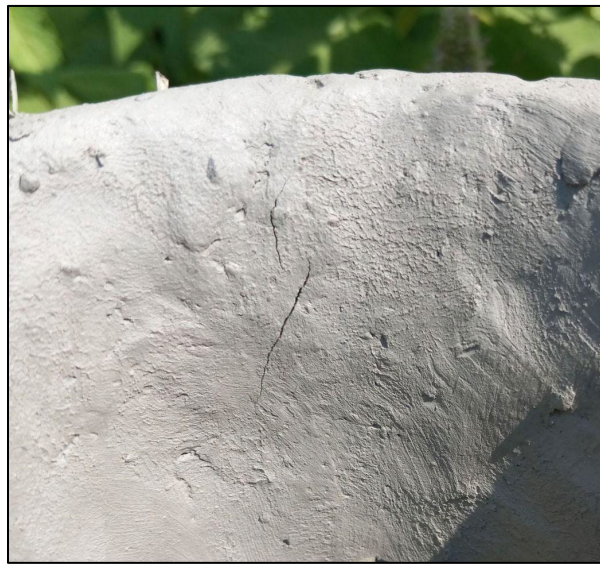
Figure 15. Detail of dried pot showing cracking.
