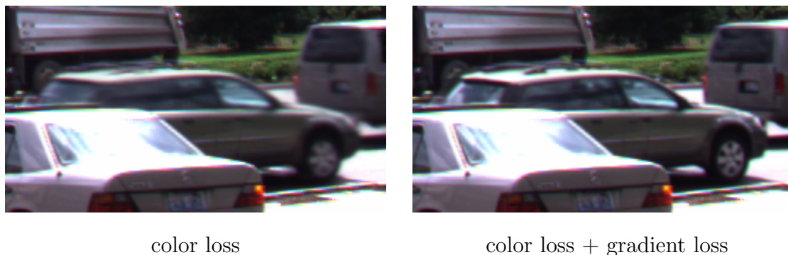
Figure 3.3: Effect of using an additional gradient loss. (a) Using the color loss alone can lead to blurry results. (b) Combining the color loss and gradient loss enables our method to produce sharper interpolation results (most noticeable in front-wheel region of the middle car).
