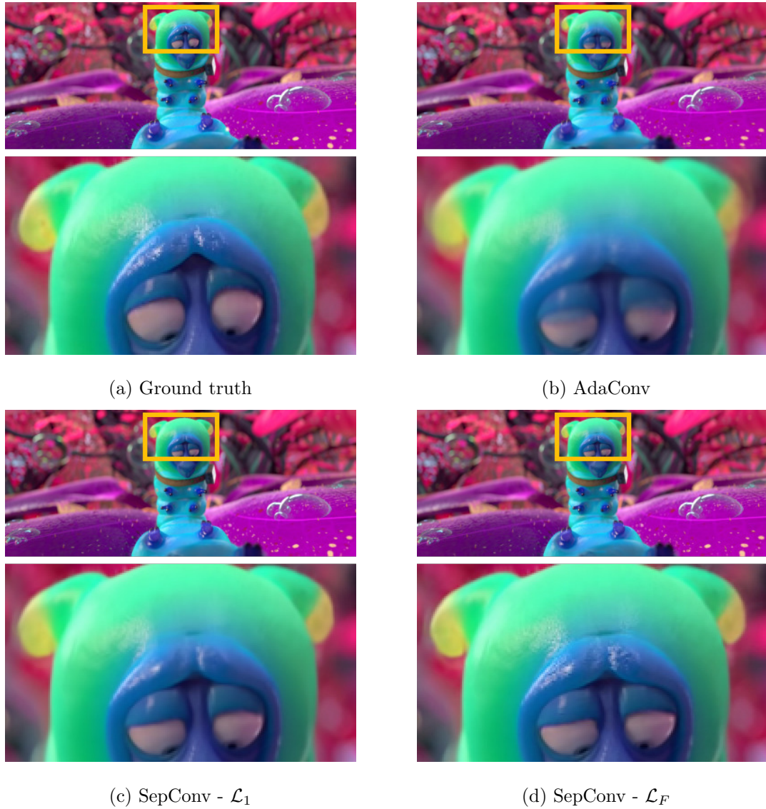
Figure 3.12: Compared to the our original AdaConv approach that utilizes 2D kernels (b), our new separable convolution methods [128], especially the one with perceptual loss (d), incorporate 1D kernels that allow for full-frame interpolation and produce higher-quality results.
