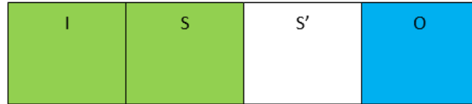
Fig. 43 Cell in green demonstrates the input cells of the output function \lambda , and the blue cell shows the output cell.
