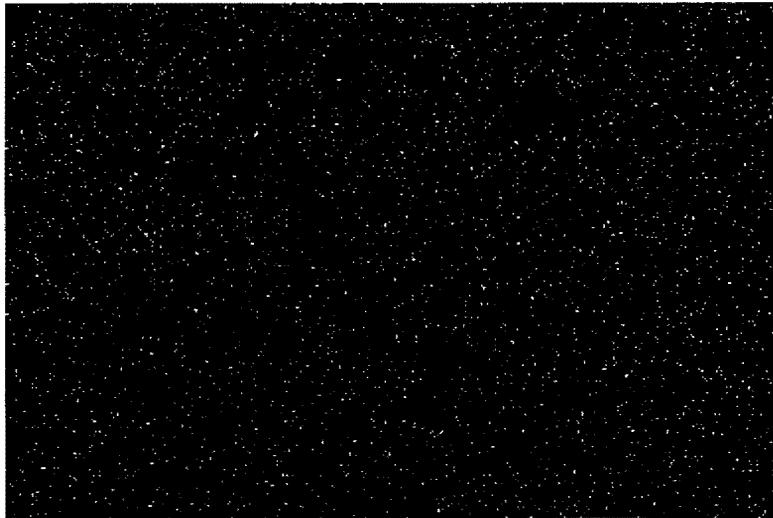
**Fig. 13** Dark frame taken with an exposure time of 500 seconds at 18° Celsius (Kodak CCD imager KAF 1600-2).
