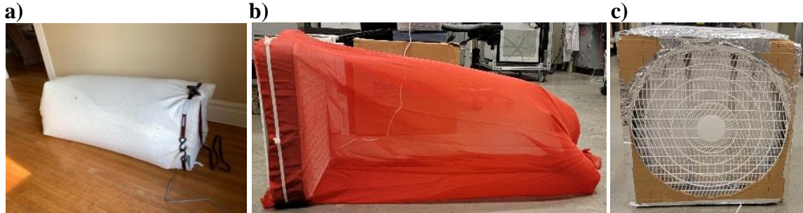
Figure 2: Image of low-cost air cleaner with a) cotton batting filter attached during the field testing, b) chiffon filter attached during laboratory testing, and c) cardboard shroud affixed during large-scale chamber testing
