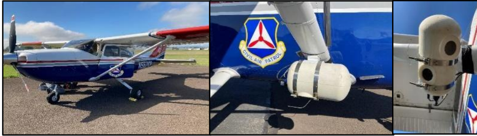
Figure 6. (A) CAP plane, (B) WaldoAir mounted on the plane wing, (C) image of sensor from below showing the two cameras.
