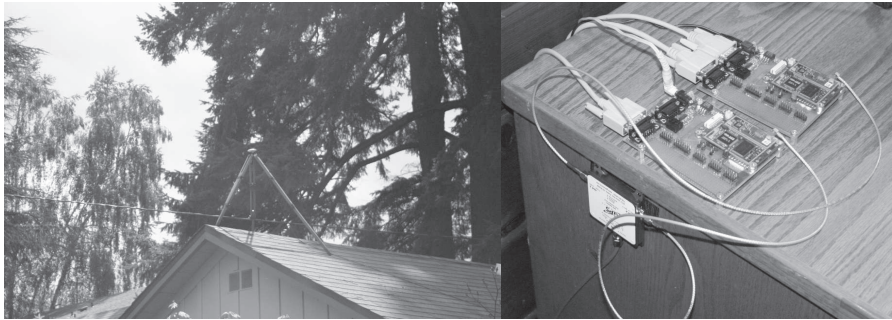
Figure A.1: Comparison testing setup: roof-mounted antenna, antenna splitter and two MG5001 receivers on development boards
