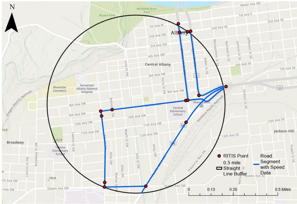
Figure 4-14 Example of Measuring Actual Speed within Buffer Around Respondent's Mailing Address
