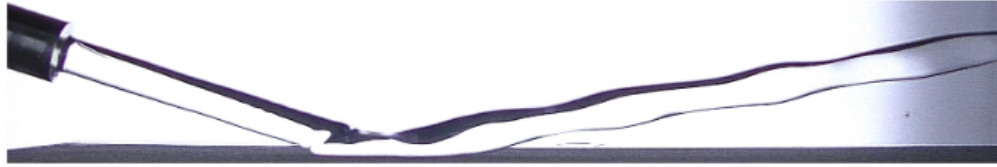
Figure 2.4: Image from a drop tower test showing a 6 mm diameter jet impacting and rebounding from a sandpaper based super hydrophobic substrate [6].
