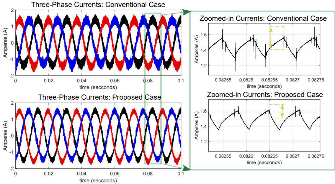
Figure 4.10: Waveforms of the three-phase AC currents with the conventional (top) and proposed (bottom) modulation strategy. [21]
