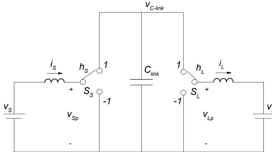
Figure 3.1: Conventional topology for a DC-DC converter example.
