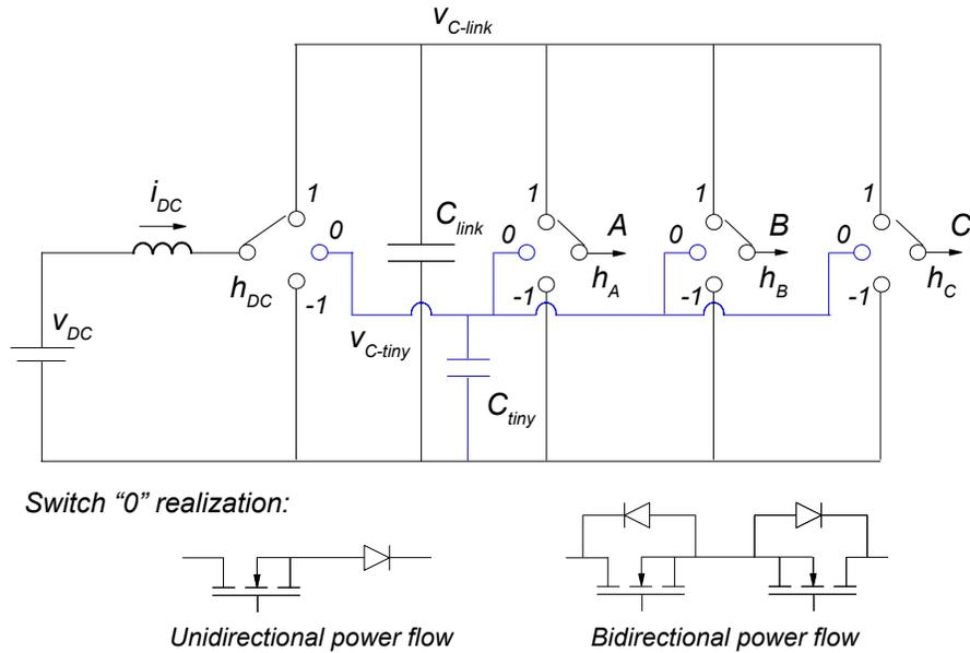
Figure 3.10: The Proposed case DC-AC three-phase topology [21].
