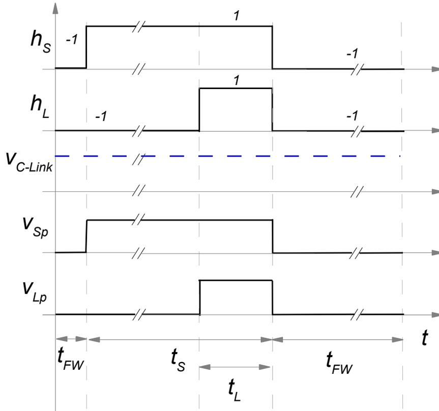
Figure 3.3: Conventional buck mode Waveforms of the switching functions ( $h_S$  and  $h_L$ ), Bulk capacitor voltage  $V_{C-link}$ , source and load-side pole voltages ( $v_{Sp}$  and  $v_{Lp}$ )
