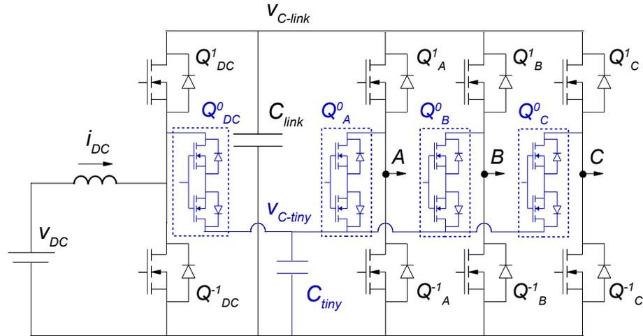
Figure 3.11: Circuit schematic for the proposed DC-AC power conversion [21].
