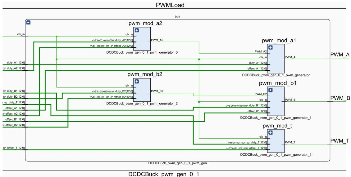
Figure 4.2: Schematic view of proposed case load side PWM generator block
