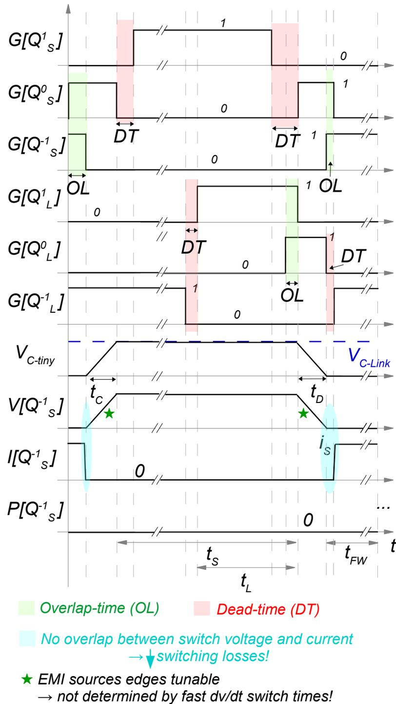
Figure 3.9: Waveforms of the gate signals of the source and load transistors ( $G[Q^x_y]$ , where  $x = -1, 0, 1$  and  $y = S, L$ ), tiny capacitor voltage ( $V_{C\text{-tiny}}$ ), and the voltage, current and power waveforms of the source-side bottom transistor ( $V[Q^{-1}_S]$ ,  $I[Q^{-1}_S]$ ,  $P[Q^{-1}_S]$ ) with buck mode of operation[21].
