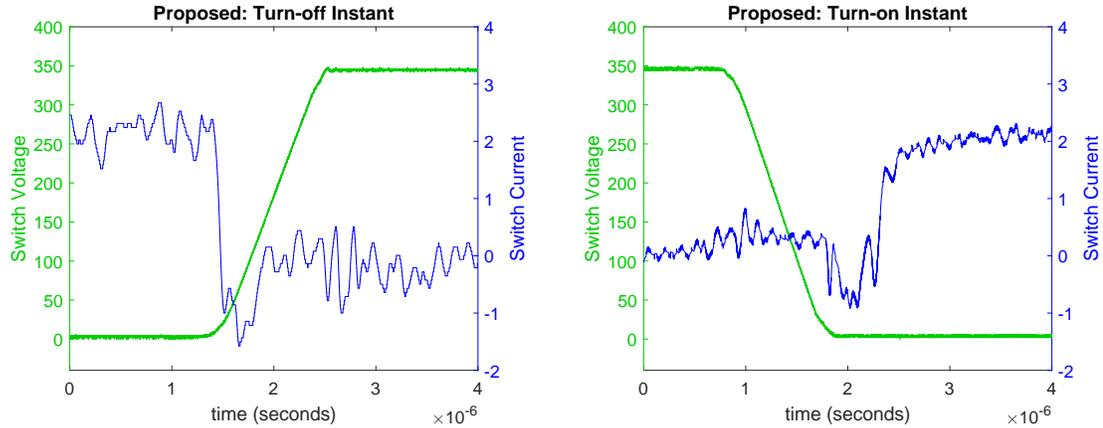
Figure 4.8: Experimentally measured switch voltage (green) and current (blue) waveforms during turn-off transition (left) and turn-on transition (right) illustrating zero-voltage switching operation on the silicon device test setup [21].
