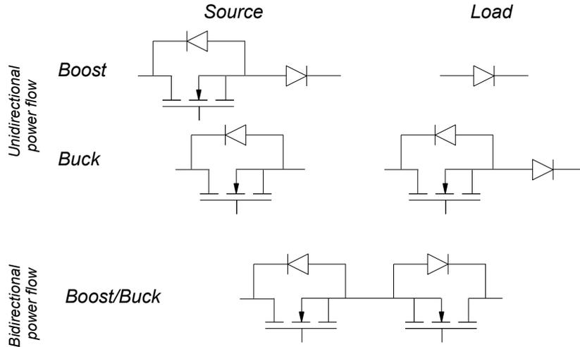
Figure 3.7: Switch realizations for the middle switch for the proposed DC-DC converter. [21]
