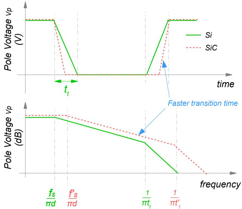
Figure 2.1: Comparing the transition time for Si and SiC devices
