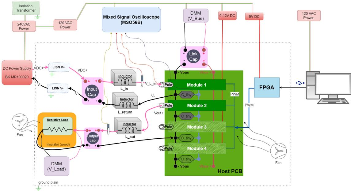
Figure 4.12: SiC DC-DC Test Setup block diagram
