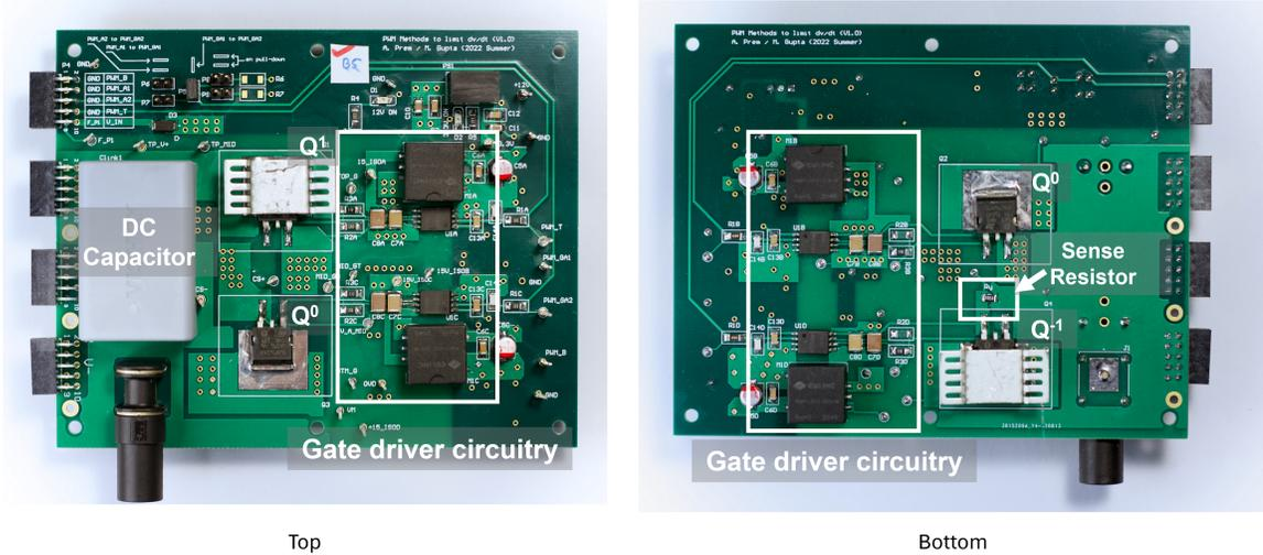
Figure 4.4: The prototype half-bridge module using Si devices
