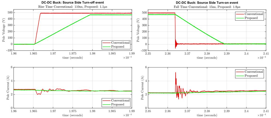
Figure 4.14: Experimentally measured  $Q_S^{-1}$  switch turn-off (left) and turn-on (right) transition with the conventional (red) and the proposed (green) approach where the voltage transition time is 110ns and  $1\mu s$  respectively. The bottom waveforms illustrate noise propagation to the pole current ( $i_S$ ) with the conventional (red) and the proposed (green) PWM method.
