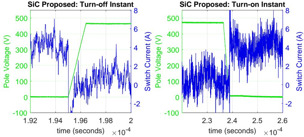
Figure 4.17: Experimentally measured switch voltage (green) and current (blue) waveforms during turn-off transition (left) and turn-on transition (right) illustrating zero-voltage switching operation on the SiC device test setup during DC-DC buck operation
