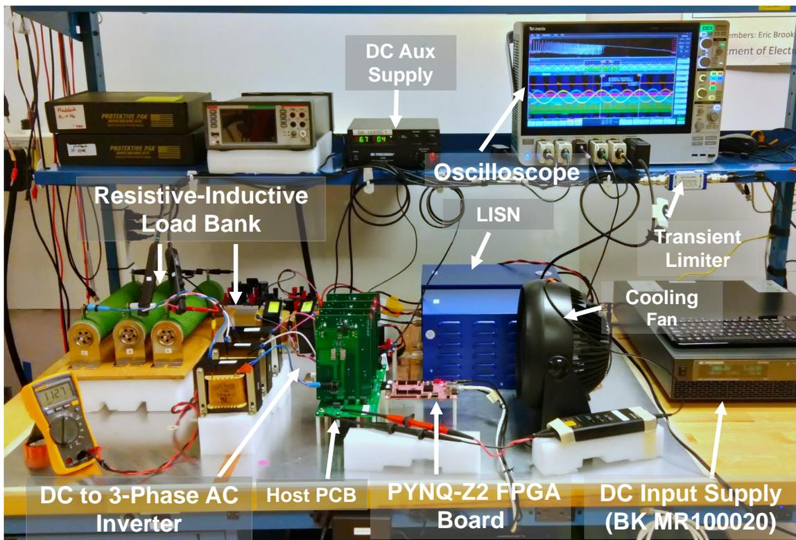
Figure 4.19: The prototype converter setup for DC to 3 phase AC topology using SiC devices
