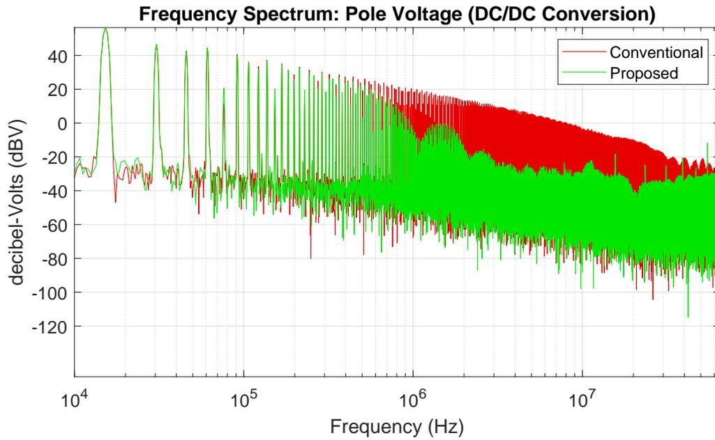
Figure 4.6: Experimentally measured frequency spectrum of the trapezoidal-shaped switch voltage (green) compared against the conventional case (red) [21].
