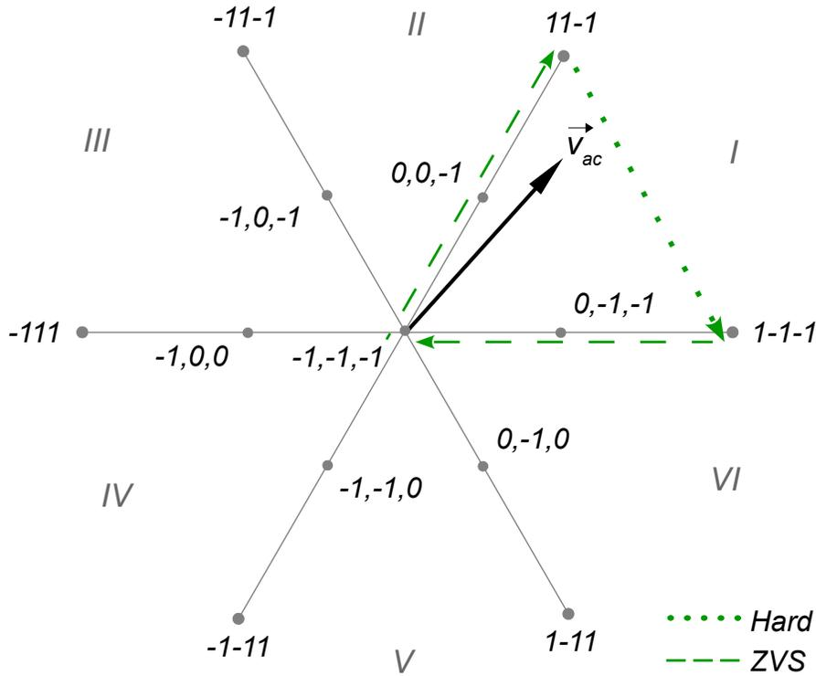
Figure 3.12: Space vector diagram for the AC inverter operation with the proposed PWM method [21].
