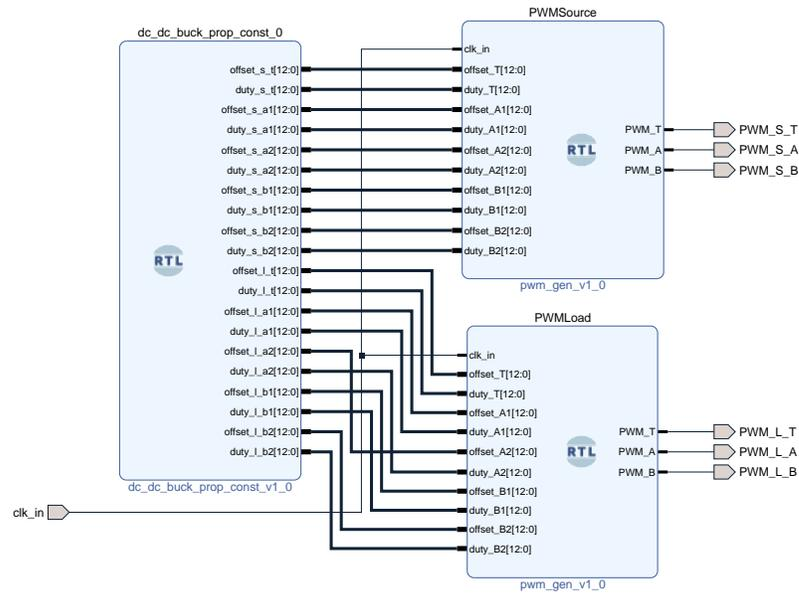
Figure 4.1: Vivado IP integrator Block Diagram for DC-DC Buck mode proposed case setup
