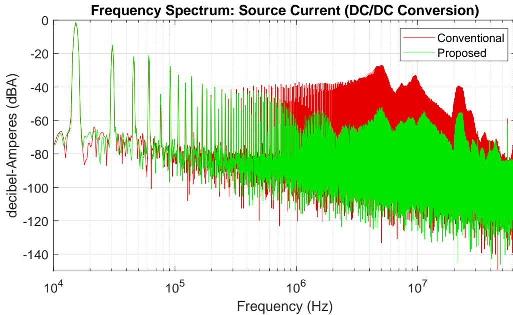
Figure 4.7: Experimentally measured frequency spectrum of the source current with trapezoidal-shaped pole voltages (green) compared against the conventional case (red) [21].
