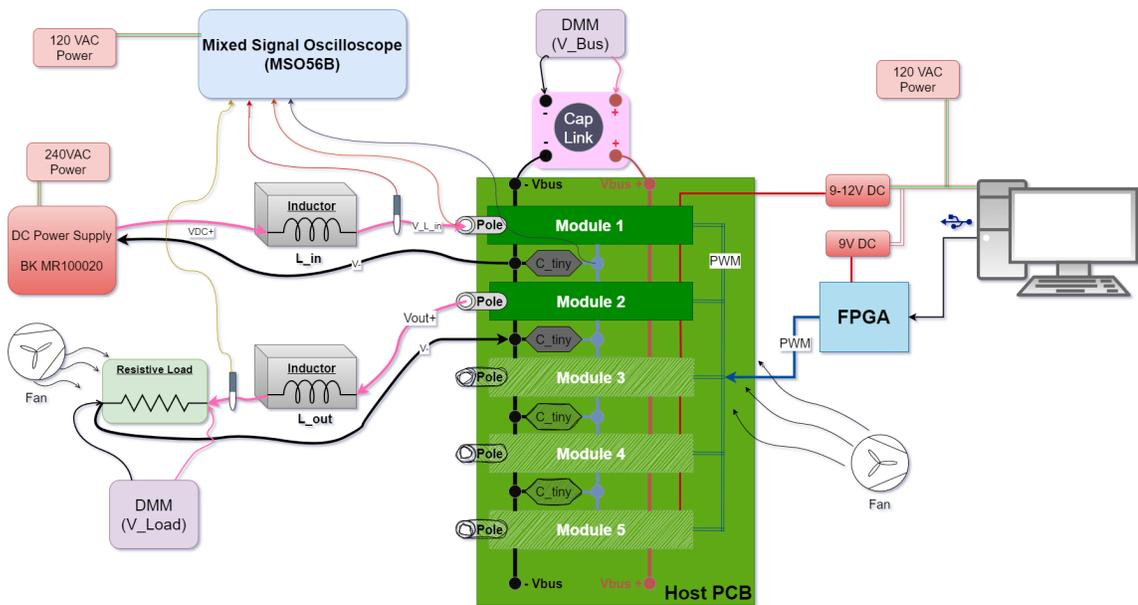
Figure 4.3: Test setup block diagram showing how the system is configured to test a DC-DC converter populated with half-bridges designed using Si MOSFETs.
