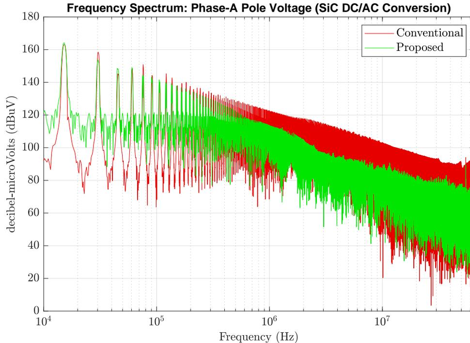
Figure 4.23: The proposed case frequency spectrum of Phase-A pole voltage (green) compared against the conventional case (red).
