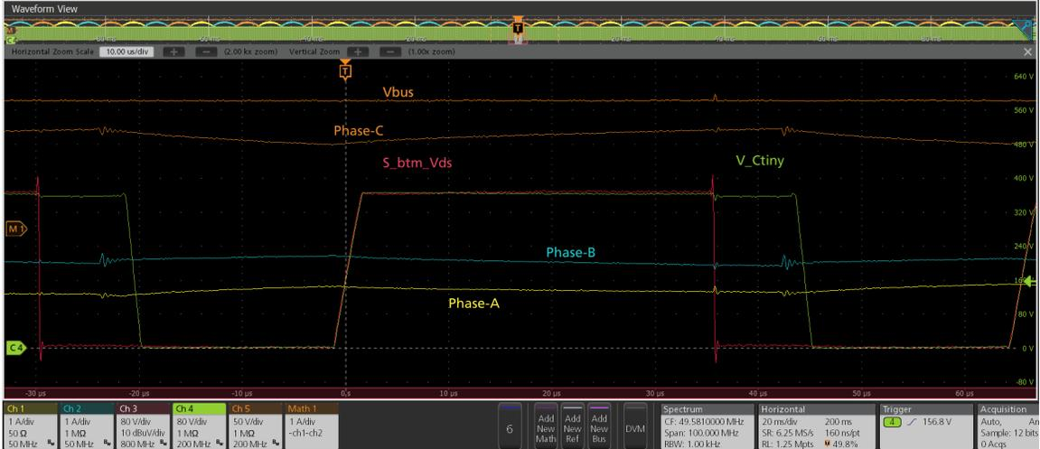
Figure 4.22: The waveform snippet obtained from the MSO for the DC-AC proposed case focusing on source side bottom switch,  $Q_{DC}^{-1}$ , the voltage on CH3,  $C_{tiny}$  voltage on CH4, the three-phase output current waveforms on CH1, CH2 and Math1, and Bus Voltage on CH5 respectively.
