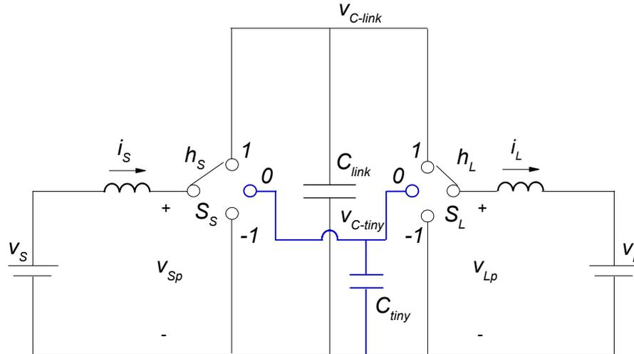
Figure 3.4: Proposed topology for a DC-DC converter example.
