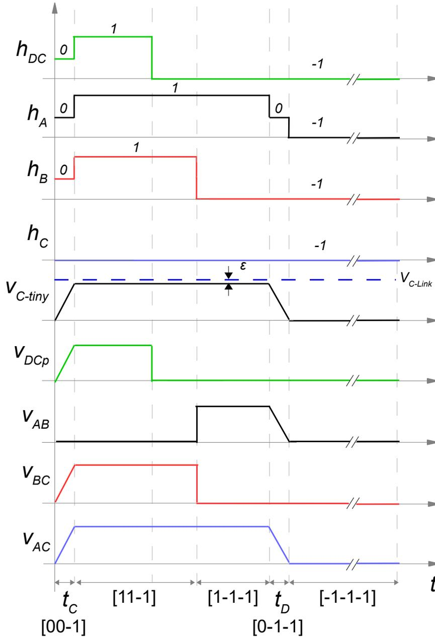
Figure 3.13: Switching waveforms for DC-AC conversion for one sector of operation[21].
