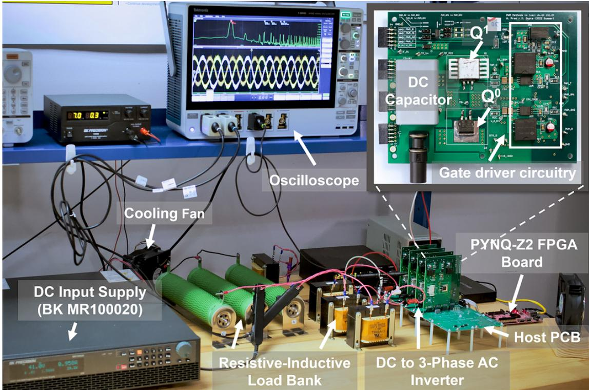
Figure 4.9: The prototype setup to test DC to 3 phase topology using Si devices [21].
