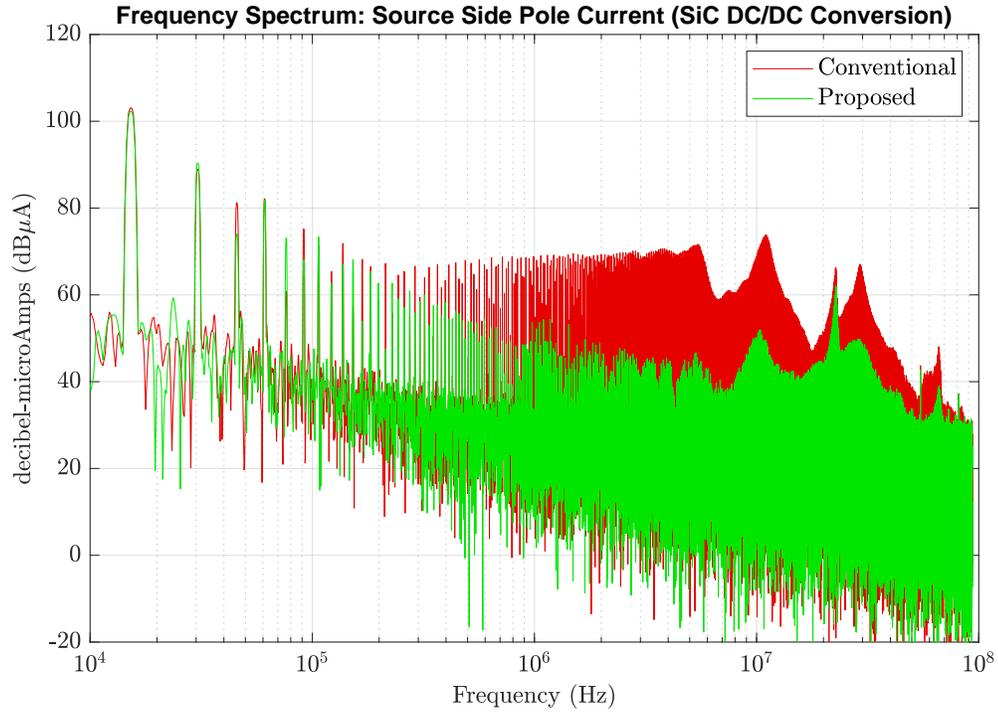
Figure 4.16: Source side pole current frequency spectrum obtained from DC-DC buck converter setup
