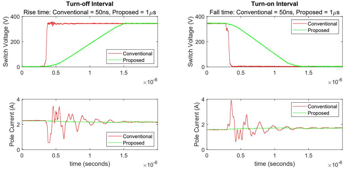
Figure 4.5: Experimentally measured  $Q_S^{-1}$  switch turn-off (left) and turn-on (right) transition with the conventional (red) and the proposed (green) approach where the voltage transition time is 50ns and  $1\mu s$  respectively. The bottom waveforms illustrate noise propagation to the pole current ( $i_S$ ) with the conventional (red) and the proposed (green) PWM method [21].
