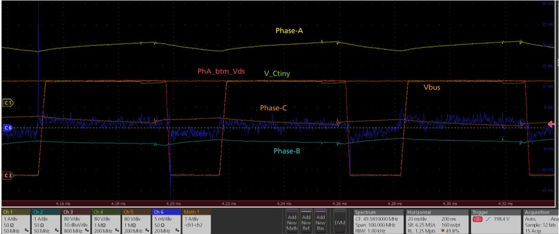
Figure 4.24: The waveform snippet obtained from the MSO for the DC-AC proposed case portraying ZVS.
