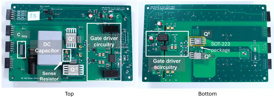
Figure 4.13: The prototype half-bridge module using SiC devices
