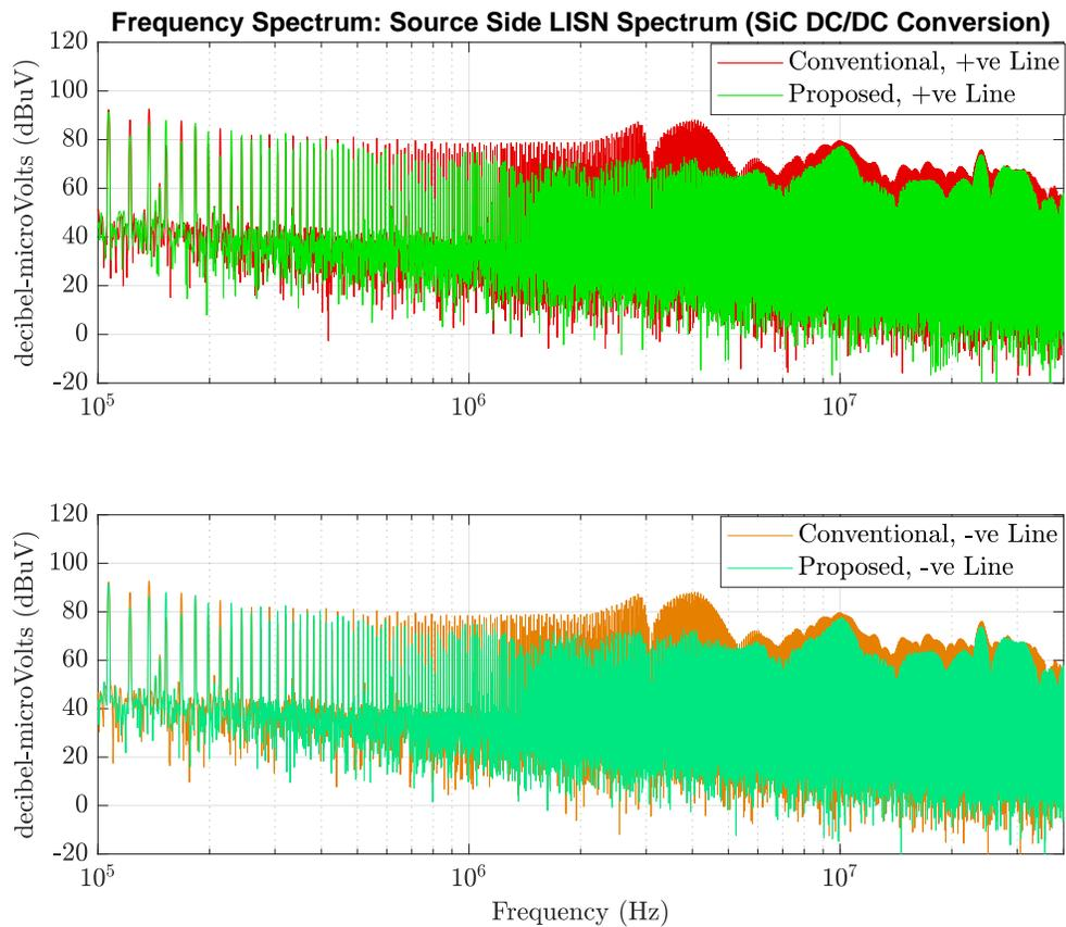
Figure 4.18: Source side LISN Spectrum comparison for DC-DC Buck operation on the SiC test setup
