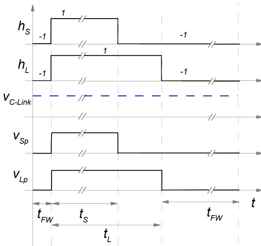
Figure 3.2: Conventional boost mode waveforms of the switching functions ( $h_S$  and  $h_L$ ), Bulk capacitor voltage  $V_{C-link}$ , source and load-side pole voltages ( $v_{Sp}$  and  $v_{Lp}$ )
