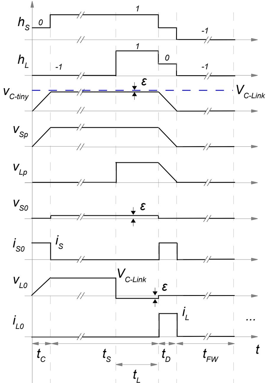
Figure 3.6: Waveforms of the switching functions ( $h_S$  and  $h_L$ ), tiny capacitor voltage ( $V_{C-tiny}$ ), source and load-side pole voltages ( $v_{Sp}$  and  $v_{Lp}$ ), and voltage, current waveforms of state "0" throws ( $v_{S0}$ ,  $i_{S0}$  and  $v_{L0}$ ,  $i_{L0}$ ) during buck mode of operation [21].
