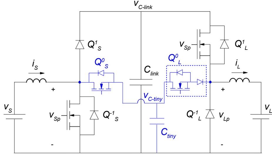
Figure 3.8: Circuit schematic of the proposed DC-DC converter with buck mode of operation and unidirectional power flow. Note that the switch additions are highlighted in blue traces [21].
