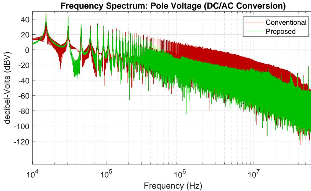
Figure 4.11: Experimentally measured frequency spectrum of the trapezoidal-shaped switch voltage (green) compared against the conventional case (red) [21].
