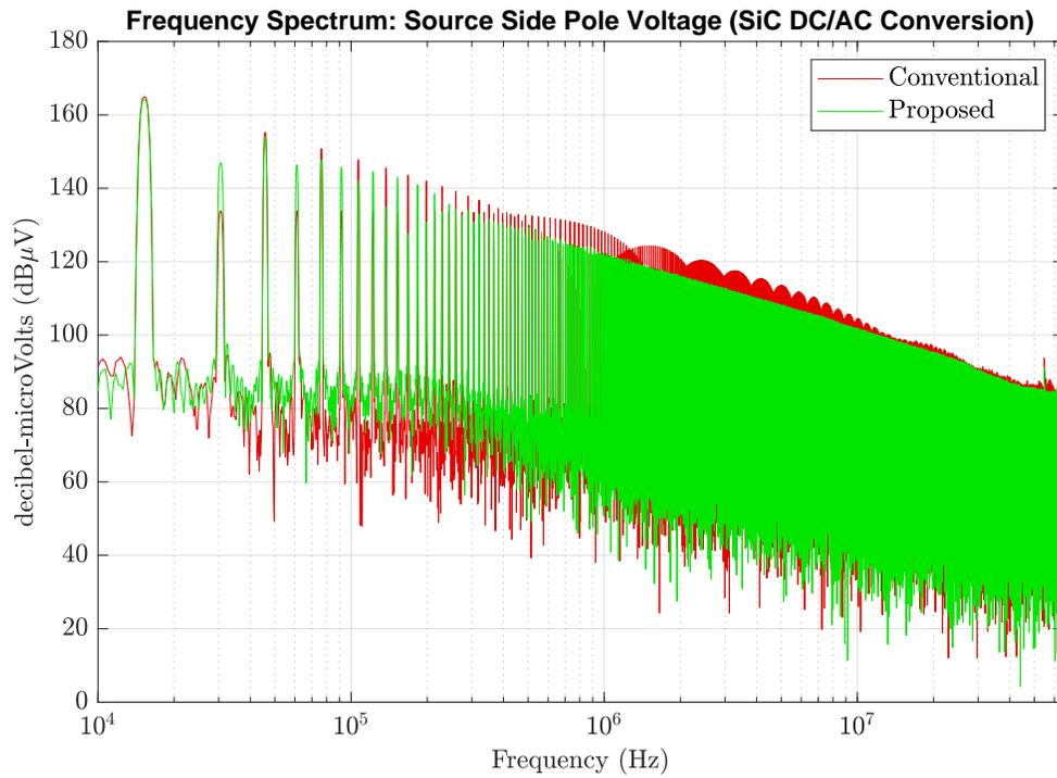
Figure 4.21: The frequency spectrum of the trapezoidal-shaped source side switch voltage (green) compared against the conventional case (red).
