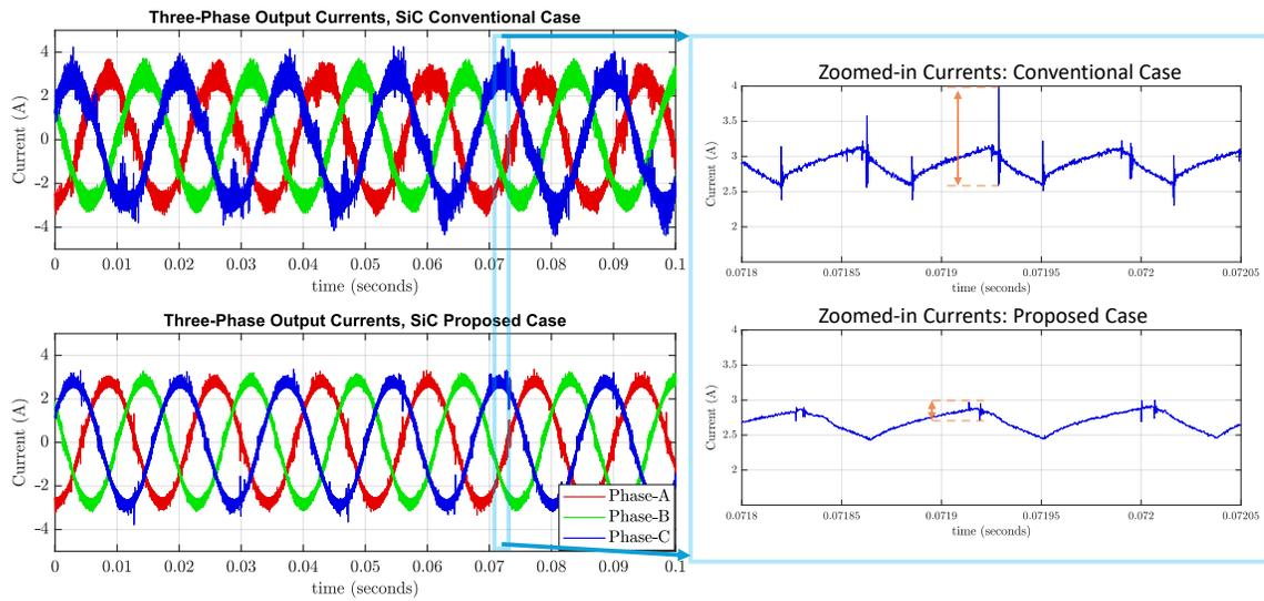
Figure 4.20: The three-phase AC waveforms with the conventional (top) and proposed (bottom) modulation strategy from SiC DC-AC converter
