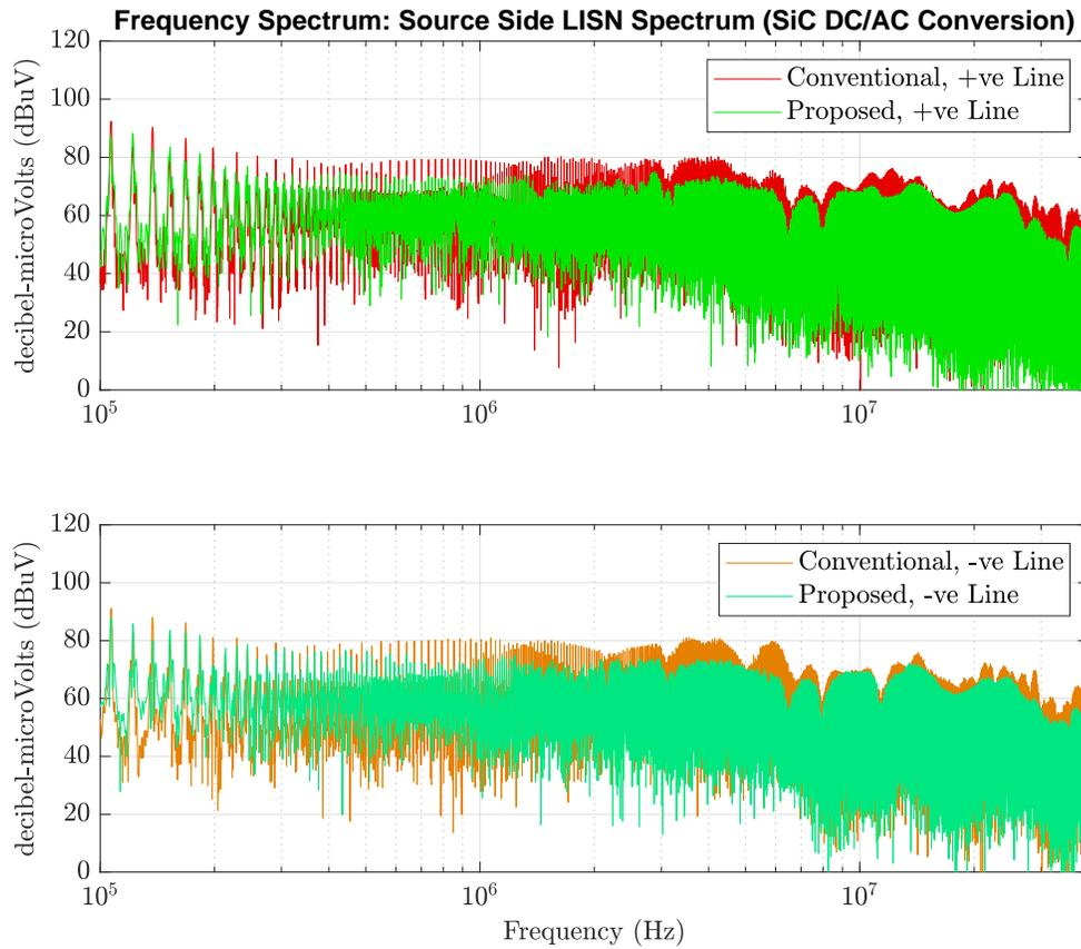
Figure 4.25: Source side LISN Spectrum Comparison for DC to three-phase AC converter
