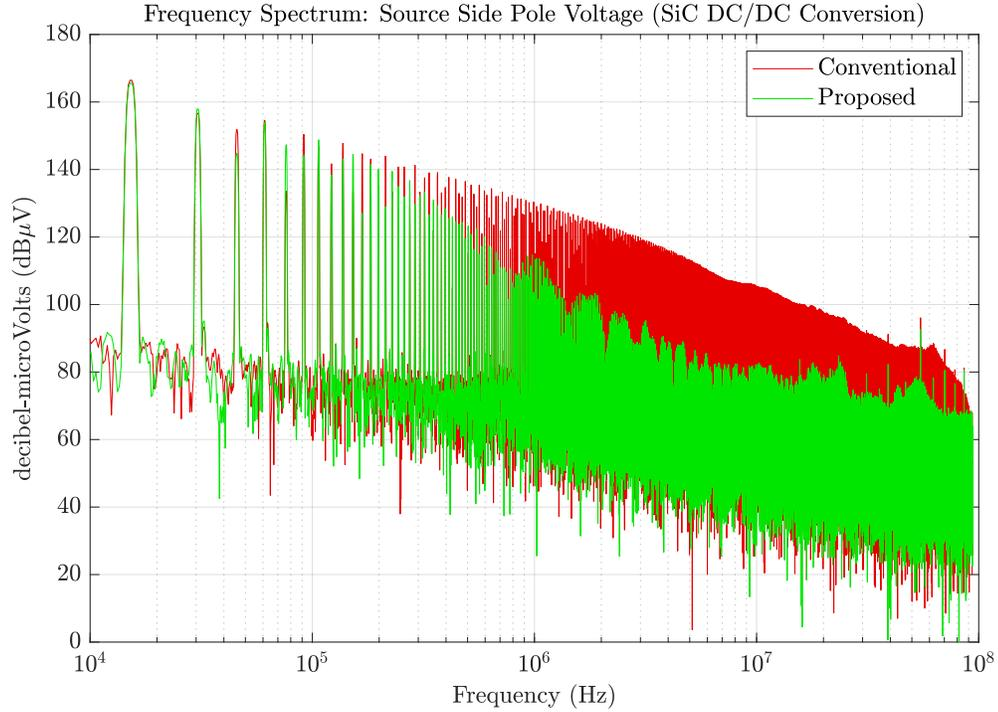
Figure 4.15: Source Side Bottom Device Pole Voltage Spectrum obtained from SiC test setup
