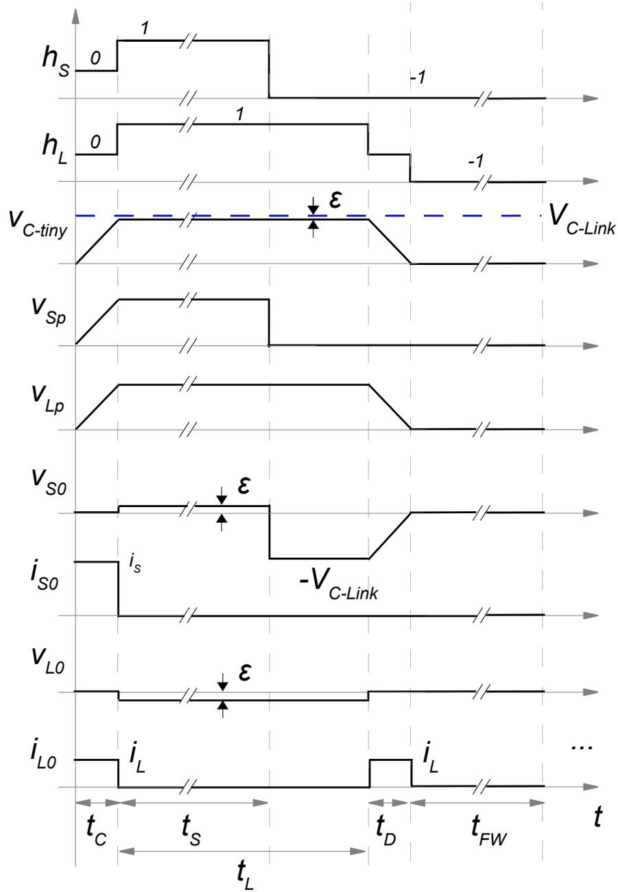
Figure 3.5: Waveforms of the switching functions ( $h_S$  and  $h_L$ ), tiny capacitor voltage ( $V_{C-tiny}$ ), source and load-side pole voltages ( $v_{Sp}$  and  $v_{Lp}$ ), and voltage, current waveforms of state "0" throws ( $v_{S0}$ ,  $i_{S0}$  and  $v_{L0}$ ,  $i_{L0}$ ) during boost mode of operation [21].
