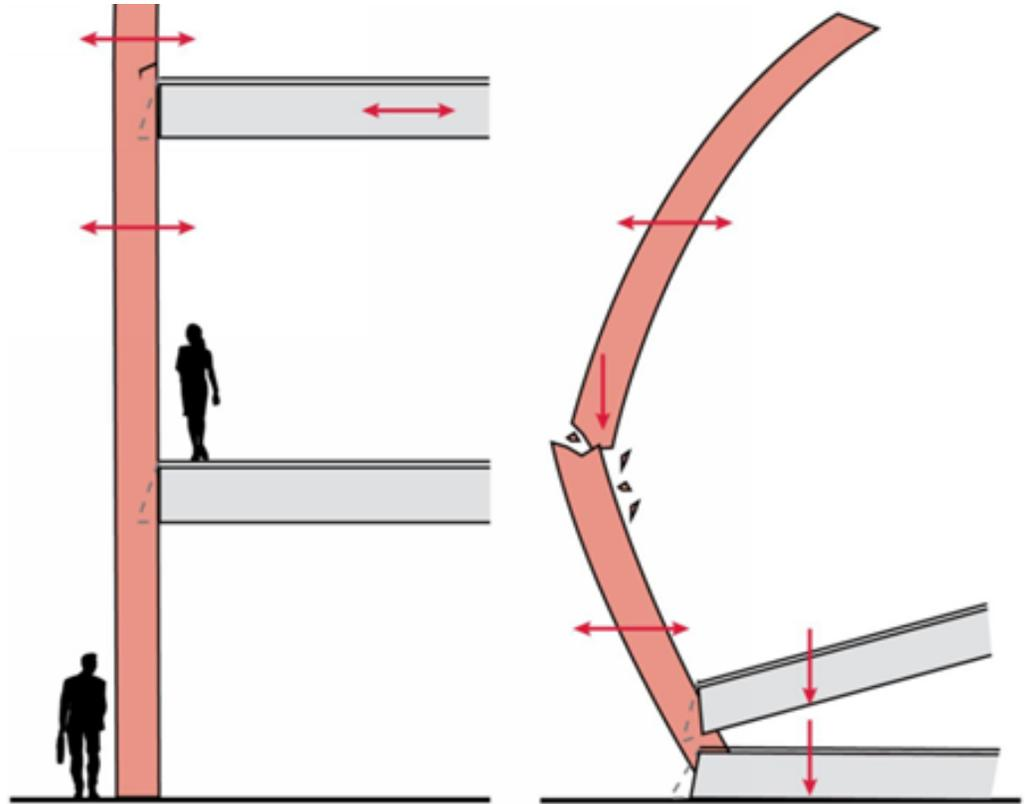
Figure 2: URM Performance in an Earthquake (Schofield, 2017)
