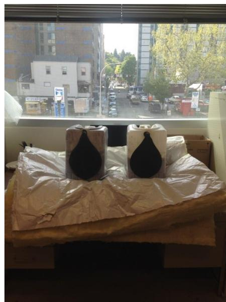
Figure 3: Placement of digesters near laboratory windows
