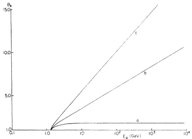
FIG. 6. Stopping number for U. *a* includes only longitudinal effect, *b* includes the sum of longitudinal and transverse effects, and *c* includes the sum of longitudinal, transverse, and spin-flip effects.
