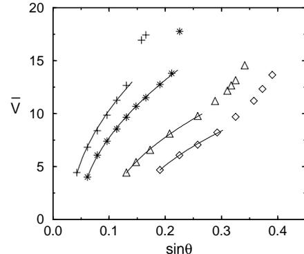
FIG. 5. Mean velocity  $\bar{V}$  (cm/s) as a function of  $\sin\theta$ . Points are experimental data taken from Ref. [4] for  $R/r = 2$  (+), 1.5 (\*), 1 ( $\Delta$ ), 0.8 ( $\diamond$ ). Solid curves are theoretical fits [Eq. (22)], ending near the last data point considered in the fit. Fitted parameters are  $(e_t, \tau) = (0.72, 33.18)$ ,  $(0.64, 21.09)$ ,  $(0.41, 10.17)$ ,  $(0.27, 7.07)$ , from left to right.
